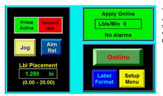
The Primary has two lamps that show which Applicator is labeling. The reason is if the line stops and both Applicators were online, without this new setup, it would be impossible to know which was the active Applicator.
