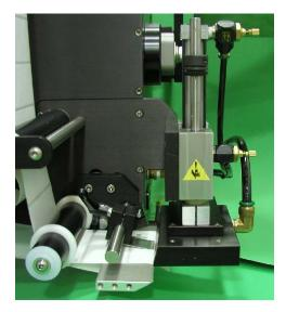
The Tamp Applicator consists of a Tamp Slide, Label Manifold, and a Label Pad. The label is fed out onto the Label Pad and is tamped within 1/8" of the labeling surface. The label is then blown off by an air blast. The Tamp Applicator has higher placement accuracy and is less dependent on product movement. **NOTE: Before proceeding, make sure you've selected Tamp in the APPLICATOR TYPE MENU on the Display. Choose one of the following types of tamping action:**
