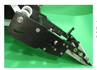
The Merge Applicator is used to apply labels to products moving on a conveyor. A label is fed onto the surface of the product at the same speed that the product is moving.
