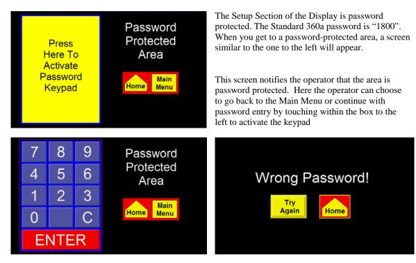
When you touch a number on the keypad, it will highlight. This is the only indication that a key was pressed since the password is not displayed. If you know you've entered a wrong number, press "C" to clear what you have and start again. "ENTER" finishes the process. If the wrong password was entered, the screen above appears. If the operator wants to try again, press the "Try Again" key. If you do not know the password, press the other key to go to the Main Menu.
