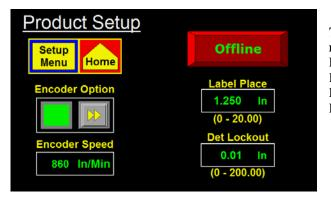
The following parameters may be changed or monitored in this section: Label Placement(s) Detector Lockout Encoder Speed (monitor) Encoder Option
