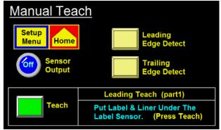
on the screen. After a couple of seconds the user is prompted to move the liner under the sensor. Move the label stock by turning the Drive Roller to place the label gap under the sensor or remove a label. Again the operator will press the Teach Key. After a couple of seconds the process is finished. The operator can return to the Label Setup Menu by pressing the "Prev Menu" Key.
