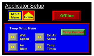
Tamp/Swing Extend and Retract Times Air Blast Time Extended Air Assist Time Web Speed Pre-Dispense Label Profile Configuration Multi-Panel Option Over Speed
