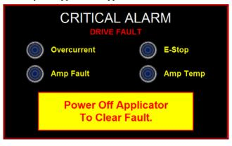
*Amp Fault* - If this occurs, there has been a failure on the Drive Board. The factory should be consulted if this occurs.
