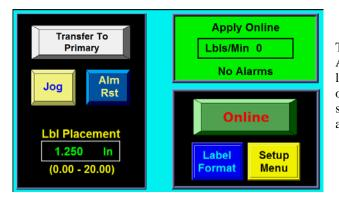
The Secondary has a new button that if this Applicator is active, you can transfer the labeling back to the Primary with less chance of missing products. Pressing this button will start the Primary labeling (if it is online) and after the Off Distance, the Secondary stops.
