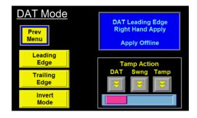
**Note:** With the Applicator Type set to DAT, jogging the Applicator will cause the Blow Valve to turn on for the Air Blast Time and a label feed. There will not be any movement from the Tamp Assembly.
