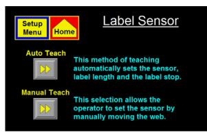
Label Sensor -Pressing this key will bring up the Label Sensor Menu. This is where the sensitivity of the Label Sensor is setup. The operator will have two choices:
