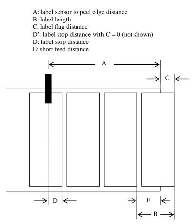
When the Multi-Panel Option is turned on, the user is prompted to go to the Label Setup Menu and perform a Label Sensor Auto Teach operation. The **Auto Teach** feature will calculate all of the dimensions shown above if the option is enabled prior to running auto teach. The operator may override these settings by measuring values B through E above and entering them via the Display. **Note: Since the Multi-Panel Apply Option is distance based, the Encoder Option must be purchased.**
