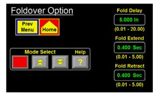
Foldover Option – Enabling this Option will allow the Applicator to control a fold station as part of the
