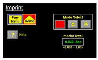
Value is now the delay the Applicator will wait before looking for the Sequence Complete Signal from the Imprinter. This delay should be close to matching the Imprinter's Dwell Time. The Help Key will also explain each Mode at the Display.
