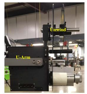
Moving by hand will take at least two people. The U-arm should be rotated down in the position shown to the left. Have a person on each side of the applicator with the one on the applicator nose side lifting only off the U-arm. The one on the unwind side (shown in the picture) will lift with one hand on the U-arm and one on the unwind shaft. This will provide enough leverage so the applicator will not tumble out of the hands of the movers.
