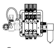
5 <u>VALVE BANK ASSEMBLY</u> SCALE: 2"=1'-0"
