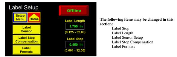
**Label Length** -The label length is defined as the feed length of the label plus the width of the gap between labels. Stated another way, it is the distance from the leading edge of one label to the leading edge of the next label. Since each application cycle moves the label length distance, it is important to enter the exact label length value. Allowed values are between 0.125-32".
