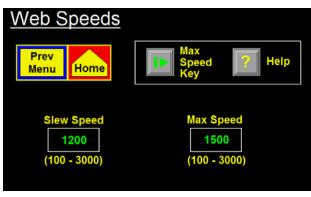
Max And Slew Speeds -The Web Speeds Menu allows access to the Max and Slew Speed values for the Applicator. Other Motion Parameters (such as Accel and Decel) are accessed thru the Special Options Menu.
