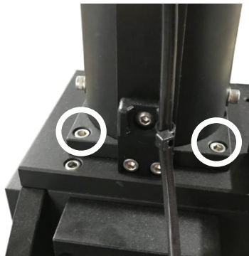
Figure 2) Guard flange and cable ties. Bolts to remove guard flange are circled
