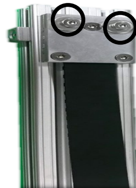
Figure 3) Stainless steel guard. Bolts to remove are circled.
