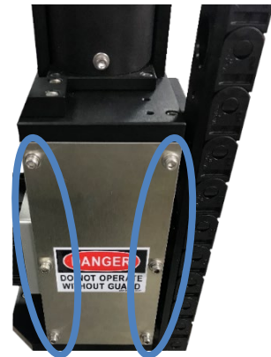
Figure 3) Stainless steel guard. Bolts to remove are circled.
