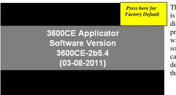
The ability to reset to factory defaults is useful when the applicator will not dispense labels due to a configuration problem. Resetting to factory defaults will bring all of the settings to something that works and adjustments can be made from there. The factory default screen can be accessed from the power-up software screen.
