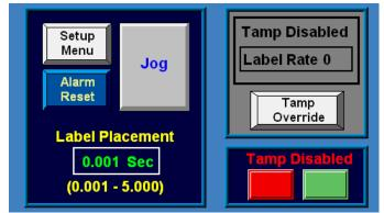
The left side of the screen will remain the same. There will always be jog, alarm reset keys and access to label placement time adjustments. Label Placement is the time from when the product detect sensor turns on until the labeling sequence starts. This is the tool used to place the label in the right position on the product.
