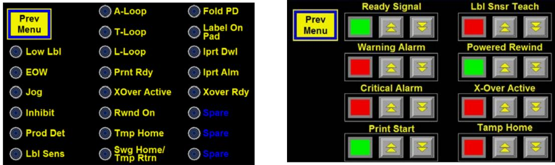
**Reset Label Sensor** –This will reset the Label Sensor to its factory values and will update the Applicator and Sensor to the Trailing Edge detection mode. After a Factory Default, the Display will go to the Label Sensor Setup Screen where the user can setup the Label Sensor again.
