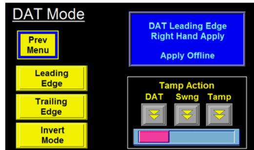
**Note:** With the Applicator Type set to DAT, jogging the Applicator will cause the Blow Valve to turn on for the Air Blast Time and a label feed. There will not be any movement from the Tamp Assembly.
