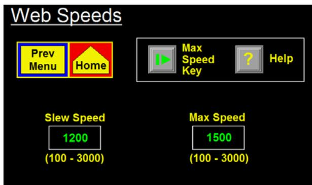
**Max And Slew Speeds** -The Web Speeds Menu allows access to the Max and Slew Speed values for the Applicator. Other Motion Parameters (such as Accel and Decel) are accessed thru the Special Options Menu.
