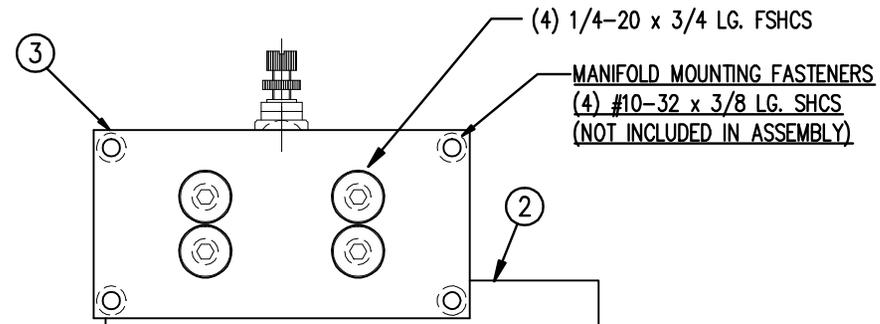
MANIFOLD MOUNTING FASTENERS
