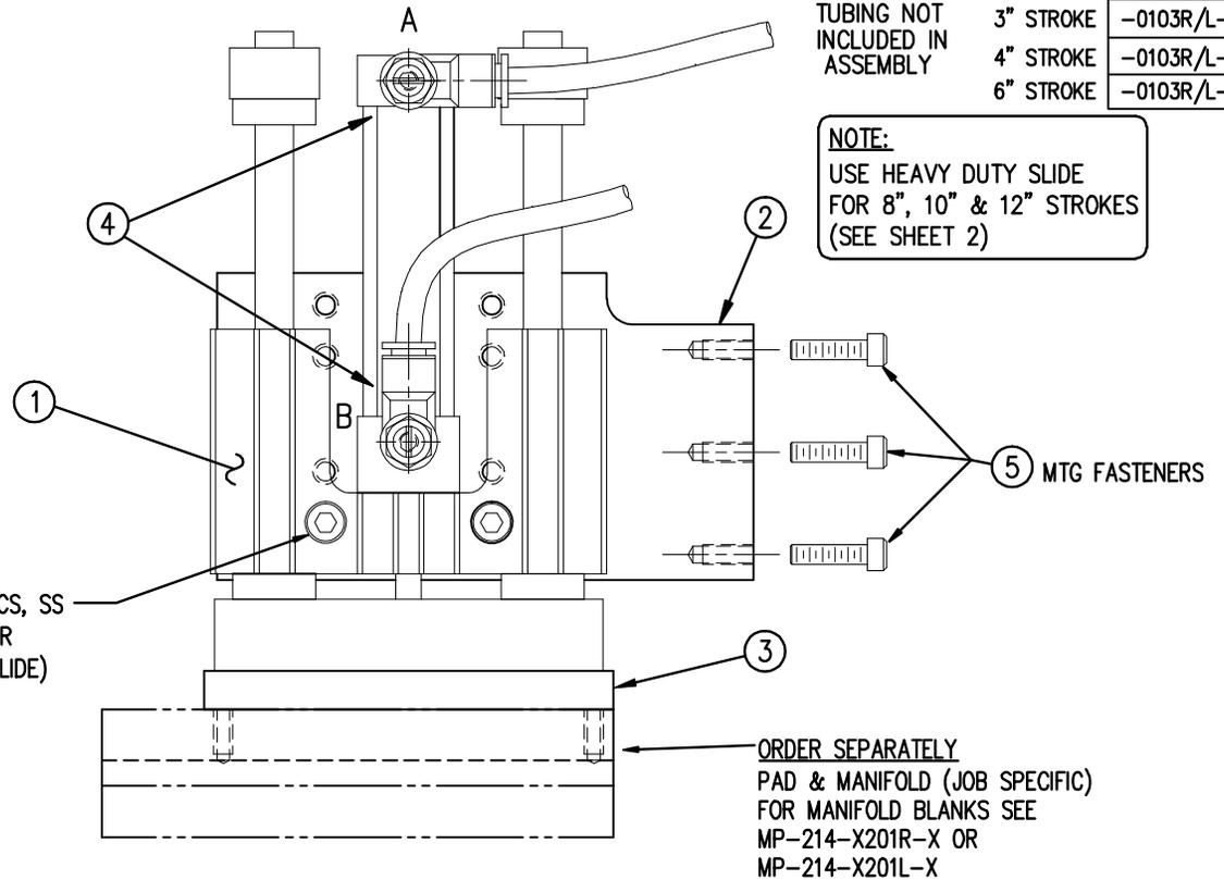
(2) 1/4-20 x 1-3/8 Lg. SHCS, SS w/HIGH COLLAR LOCK WASHER (INCLUDED WITH STANDARD SLIDE)
