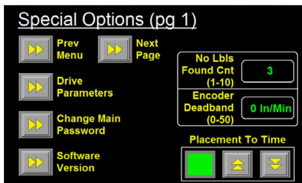
**Placement To Time** – This Option only appears if the Applicator Type is a Merge and the Encoder is turned on. You will use this when labeling in a Wrap Station that is equipped with an Encoder. This way the Applicator will dispense its label at the Encoder Speed but the start of the labeling sequence will not be dependent on the Wrap Belt position but instead will be time-based. This is good since the belt runs at a different speed than the conveyor, which is handling the product.
