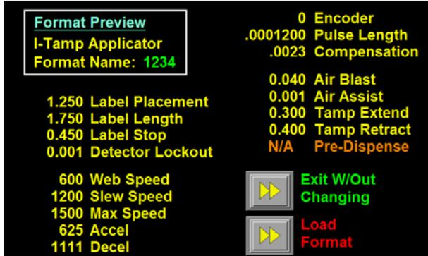
Pressing the View/Load Key will not immediately load the Format but will allow the operator to view the values within that Format. After reviewing the values, the operator may press "Load Format" to load the Format. If the wrong format was selected, the operator can press the "Exit W/Out Changing" key.
