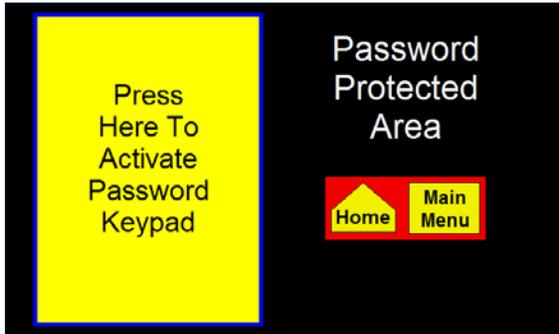
The Setup Section of the Display is password protected. The Standard 360a password is “1800”. When you get to a password-protected area, a screen similar to the one to the left will appear.
