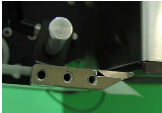
**Note: The top of the Peel Edge should be slightly higher than the bottom surface of the Label Grid. If a label on the Grid will slide back onto the Peel Edge, the Peel Edge is too low.**
