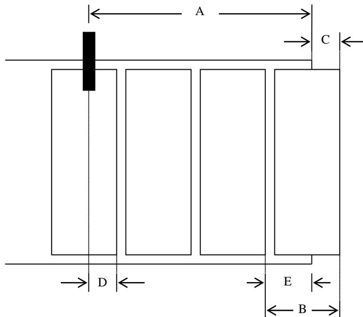
When the Multi-Panel Option is turned on, the user is prompted to go to the Label Setup Menu and perform a Label Sensor Auto Teach operation. The **Auto Teach** feature will calculate all of the dimensions shown above if the option is enabled prior to running auto teach. The operator may override these settings by measuring values B through E above and entering them via the Display. **Note: Since the Multi-Panel Apply Option is distance based, the Encoder Option must be purchased.**
