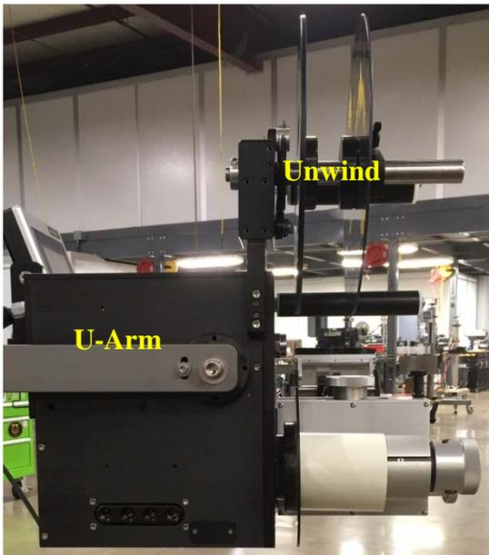
Moving by hand will take at least two people. The U-arm should be rotated down in the position shown to the left. Have a person on each side of the applicator with the one on the applicator nose side lifting only off the U-arm. The one on the unwind side (shown in the picture) will lift with one hand on the U-arm and one on the unwind shaft. This will provide enough leverage so the applicator will not tumble out of the hands of the movers.
