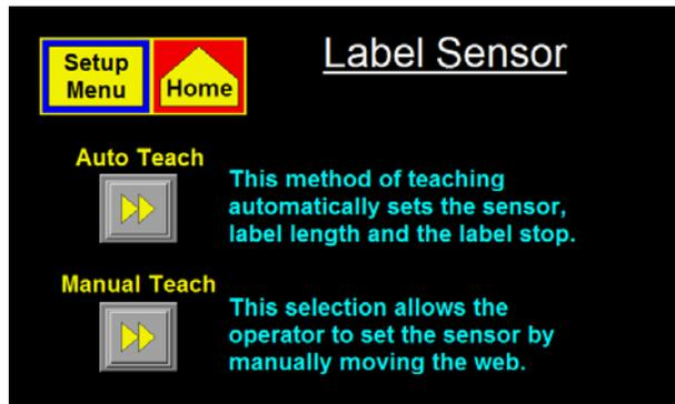
**Label Sensor** -Pressing this key will bring up the Label Sensor Menu. This is where the sensitivity of the Label Sensor is setup. The operator will have two choices:
