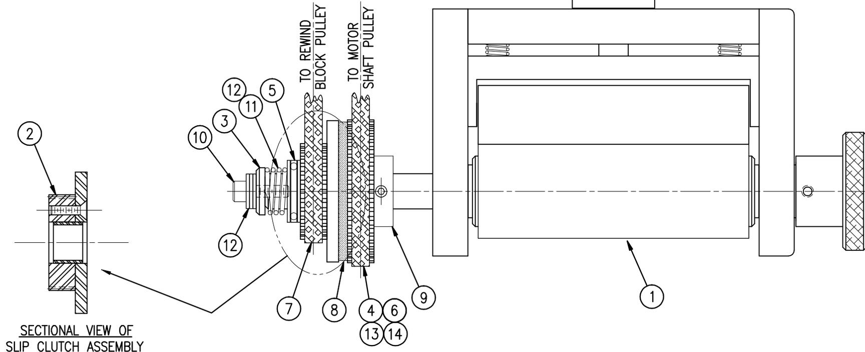
SECTIONAL VIEW OF SLIP CLUTCH ASSEMBLY
