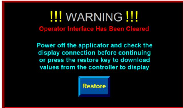
Typically, this situation occurs when the Display Cable is loose or unplugged.
