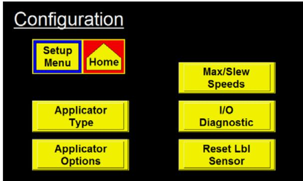
The Configuration Menu provides access to Applicator: Type Setup, Options, Motion Parameters, Diagnostics, and the Label Sensor reset function. The Applicator Setup may be monitored or changed by accessing the various submenus.
