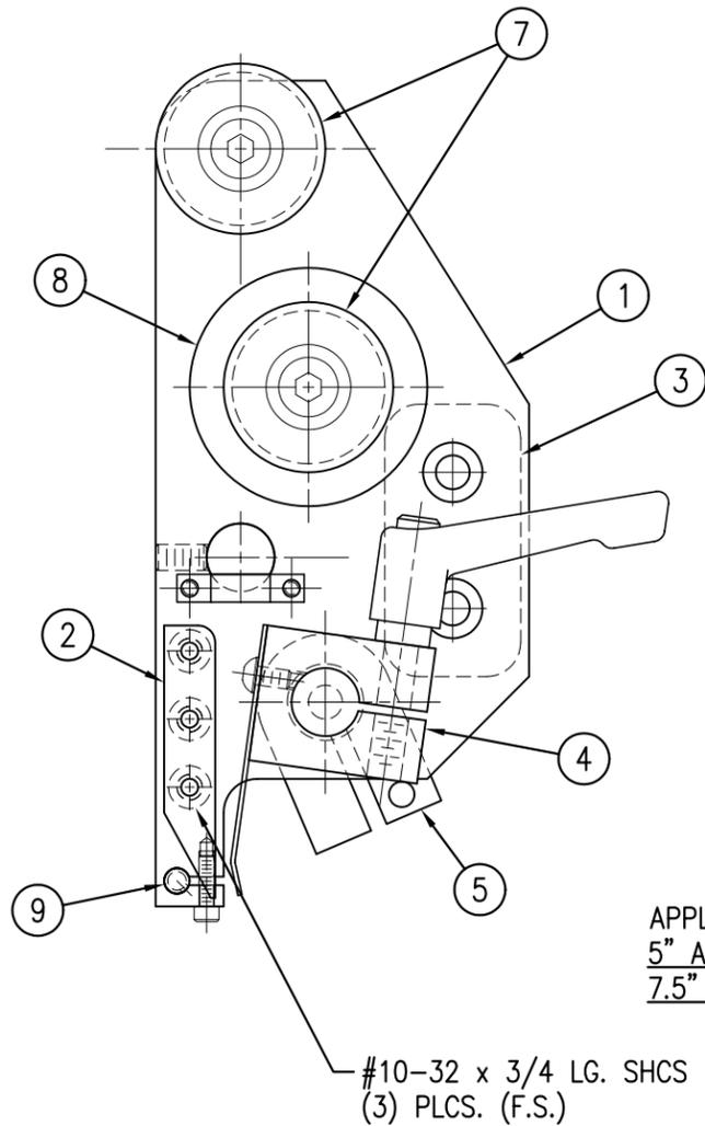
APPLY (1) STRIP OF UHMW TAPE TO PEEL EDGE ②
